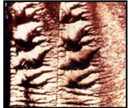
Microscopic toolmark comparison.
